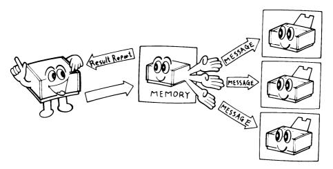
The message is stored in the memory of the broadcasting transmitter and transmitted to each designated receiver in turn.
